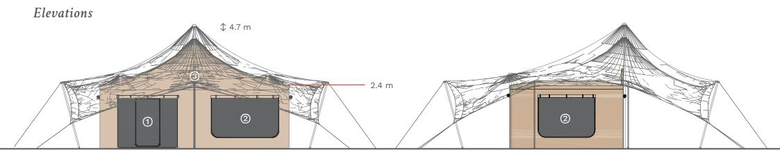
① door 2500 x 2100 mm, ② window 2500 x 1700 mm, ③ window 1500 x 600 mm, ④ door 1200 x 2100 mm, ⑤ window 1200 x 600 mm
