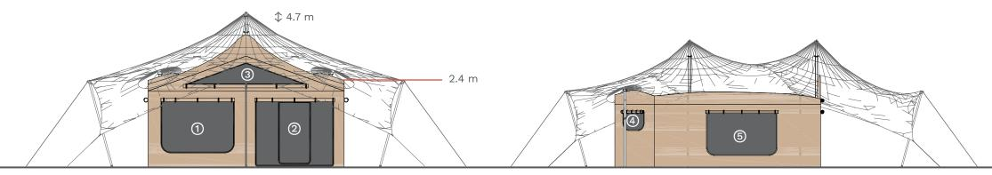
① window 2500 x 1700 mm, ② door 2400 x 2100 mm, ③ window 3700 x 700 mm, ④ window 1200 x 600 mm, ⑤ window 2700 x 1700 mm
