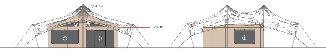
① window 3000 x 1700 mm, ② door 3000 x 2100 mm, ③ window 2000 x 600 mm, ④ window 1500 x 600 mm, ⑤ window 1200 x 1700 mm
