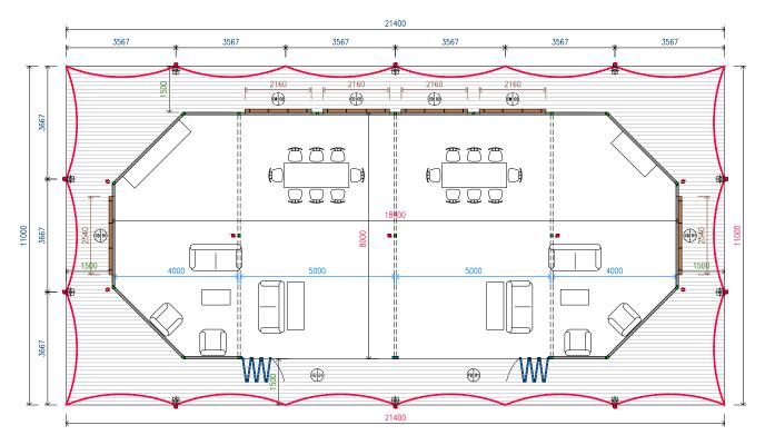
THE STRETCH TENT ROOF: 770gr Tentickle Tentflex, fire-retardant, waterproof, UV repellent, anti-microbial, highly tensile, Teflon-coated polyester stretch. The outside has a smooth, matt finish with a water-repellent lotus effect. The inside of the fabric has a natural flow and a soft, organic feel – not requiring any further draping. The fabric reflects light very effectively and offers a great canvas for spectacular lighting concepts.
